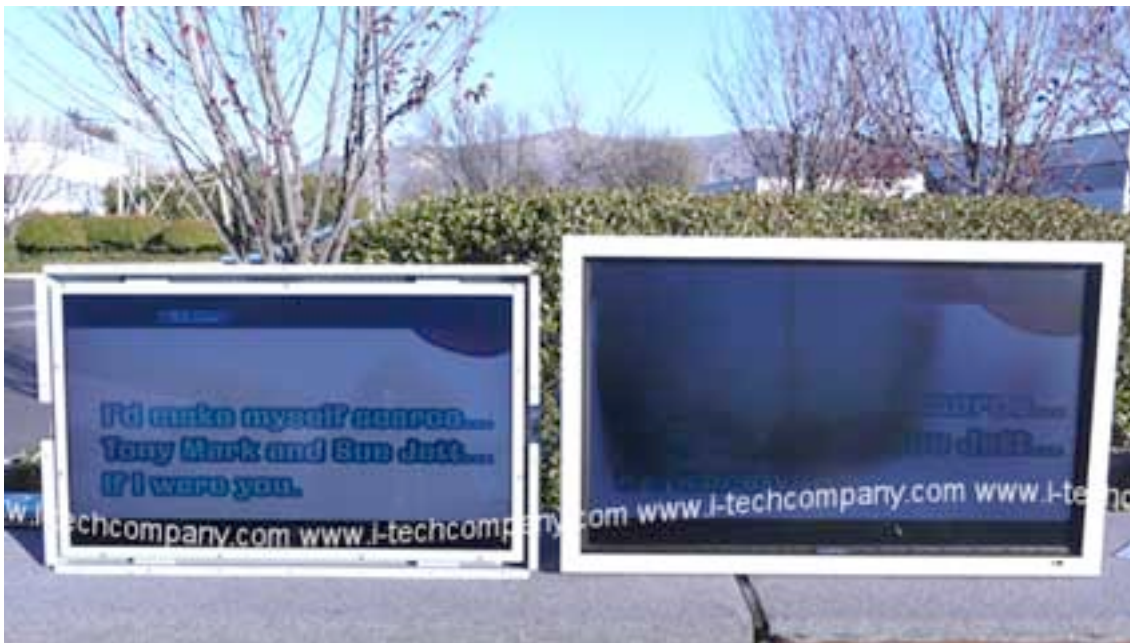
Comparison between Transflective (Left) and Britelite (Right) in sunlight
